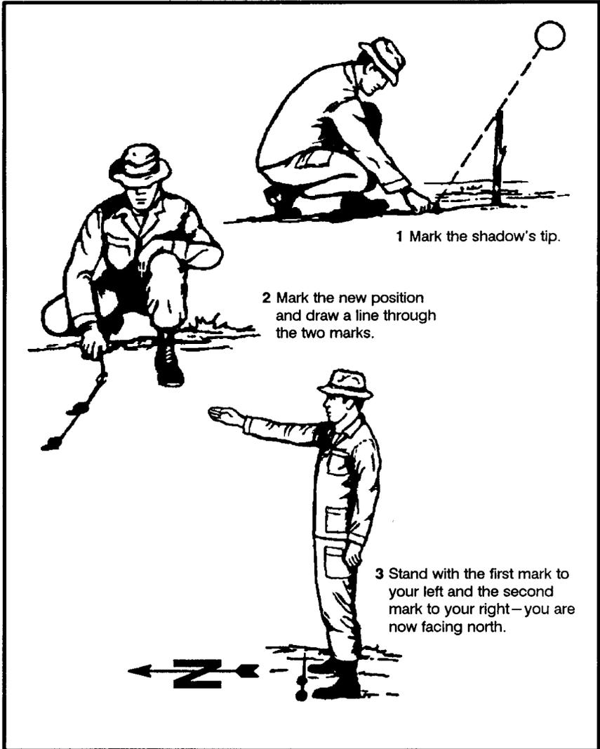
**Figure 18-1. Shadow-tip method.**
